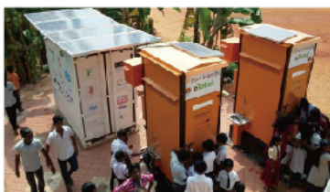
NEWgenerator 100 v.1 (white unit) undergoing field-testing at a school in Kerala, India. The orange units are Eram eToilets serving as front-end units.
